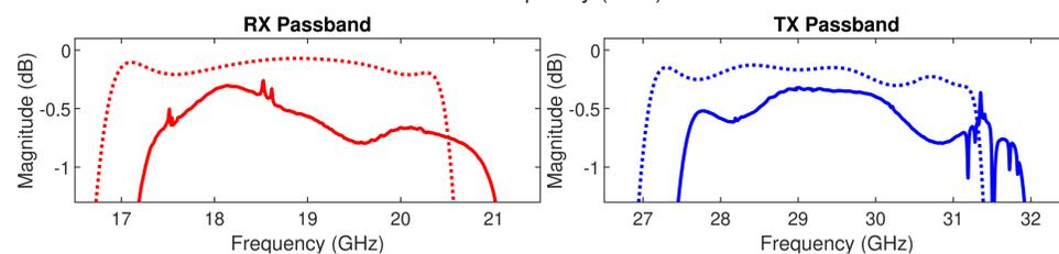
Comparison between processed measurements and simulation results
