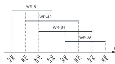
Waveguide operating frequency ranges
