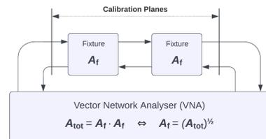
Unterminating with 2x-thru measurement
